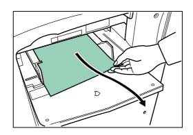
2 If the jammed paper remains at the MP tray, pull up the lever and remove the jammed paper.
